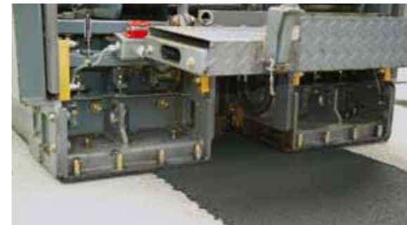
System for pave width reduction allows minimum width of 0.5m.
