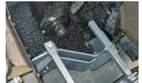
System for infinitely variable pave width reduction.
